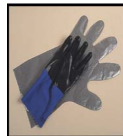
Post-accident tests showed that pairing SilverShield and neoprene gloves is the only guard against dimethylmercury.
