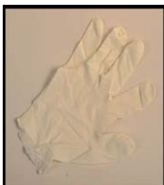
Disposable latex gloves gave Wetterhahn needed dexterity. No one knew that dimethylmercury soaks through them.
